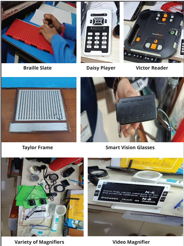
Figure-1: Some of the assistive technologies used by students in classroom and rehabilitation training.
